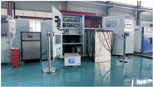
图2 采用高压数字电桥对电容器样品进行容值损耗测量 Fig.2 Using high-voltage digital bridge to measure capacitance loss of capacitor samples
